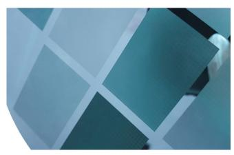
Fig 1: Wafer with laser OCF test fields
