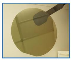
Picture of an Engineered SiC substrate
